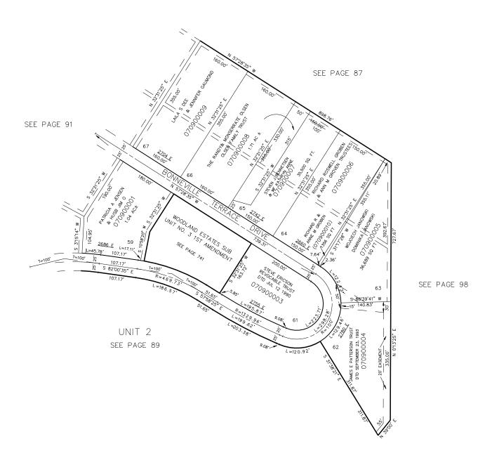
10' UTILITY & DRAINAGE EASEMENTS EACH SIDE OF PROPERTY LINES AS INDICATED BY DASHED LINES EXCEPT AS OTHERWISE SHOWN.
